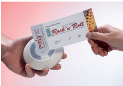
**Fig. 4. Radio-activated smart tickets provide automatic admission**
